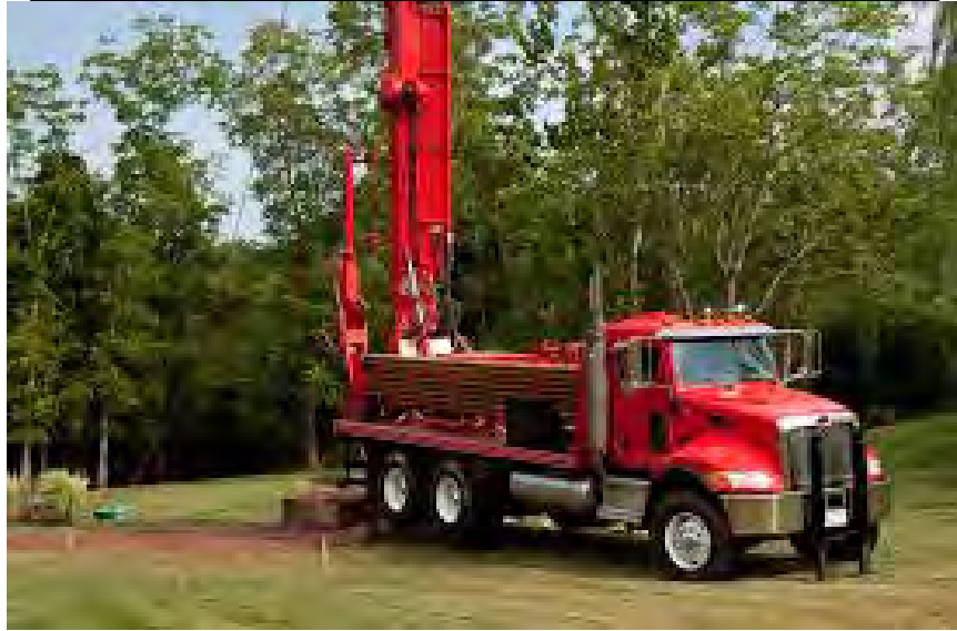
A typical well-drilling truck rig.
