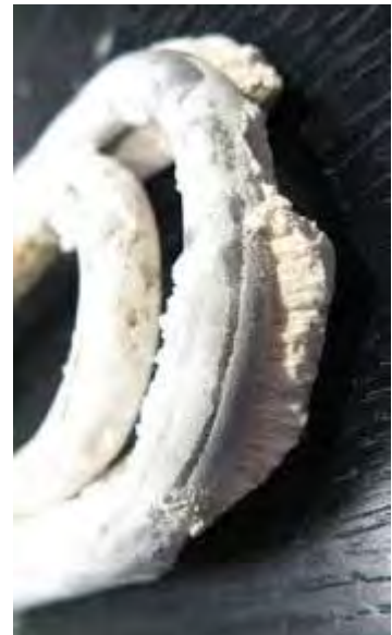
Calcification of Electrodes
